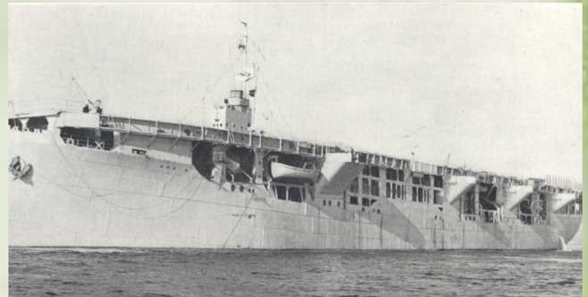
DOWN CAME THE BRIDGE, the funnel. When she was flat, they laid a deck on her.
