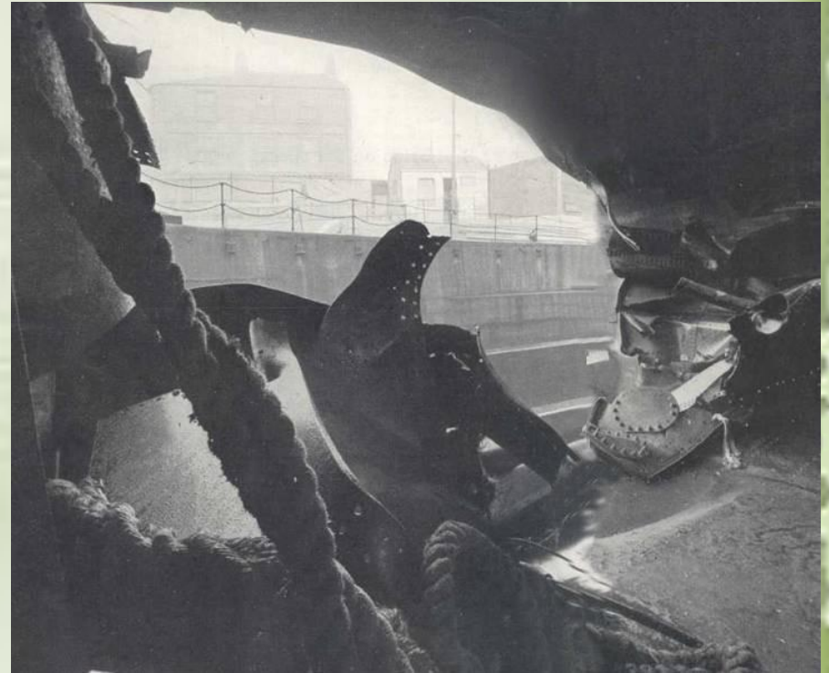
EDGED WITH CONTORTED METAL, this cavern is where a torpedo struck the Atheltemplar. Her crew got her home, the ship repairers healed her wound and made her seaworthy again. To save a ship in war time is everything.
