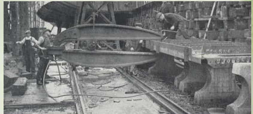
THE LOBSTER CLAWS of the hydraulic riveter, a machine used to fabricate work.
