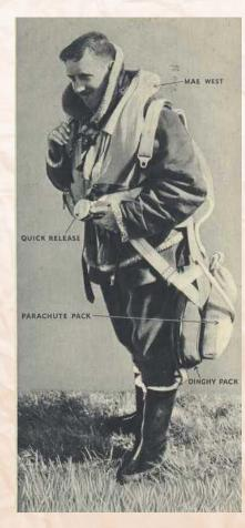
Right: Equipment for safety. The dinghy pack, 15" square by 3" thick, contains self-inflating dinghy, sea-anchor, rations, signals, repair kit, baler, cigarettes.
