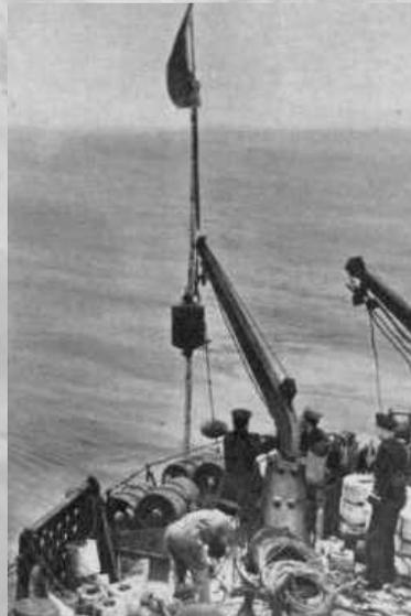
**MARKING THE SWEEP CHANNEL.** Behind the last of the sweepers comes a special vessel, the "danner." She lays dan-buoys, seen here on deck, along the limits of the safe area.
