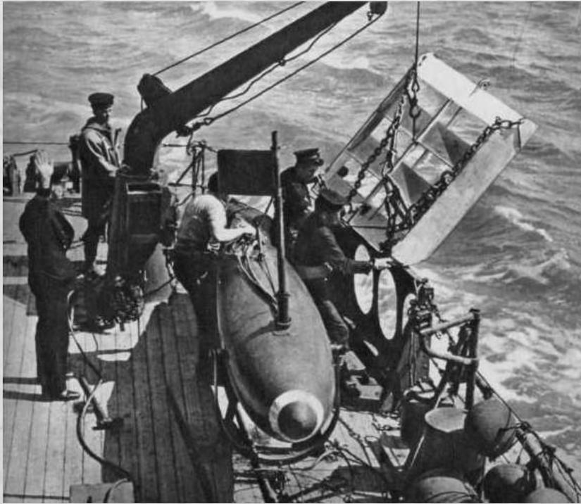
*"OUT SWEEP." Above, the float with its flag is ready on its chocks. The otter is being lowered from the davit.*
